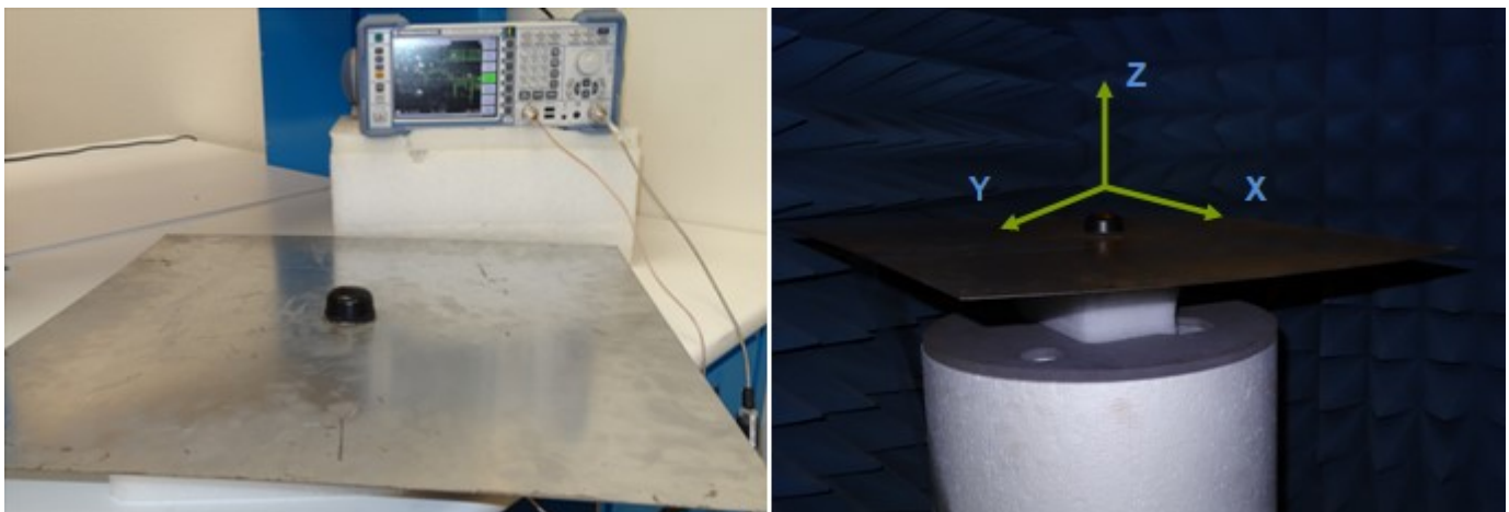
Figure 1. Impedance measurement (left hand) and efficiency, gain, radiation pattern measurements (right hand).
